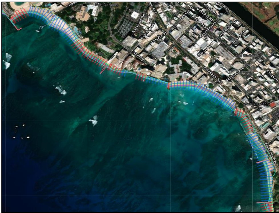
Figure 11. Historical Shoreline Change Maps. The transects alongshore represent historical erosion rates (ave feet/year) red is erosion, blue is accretion.
