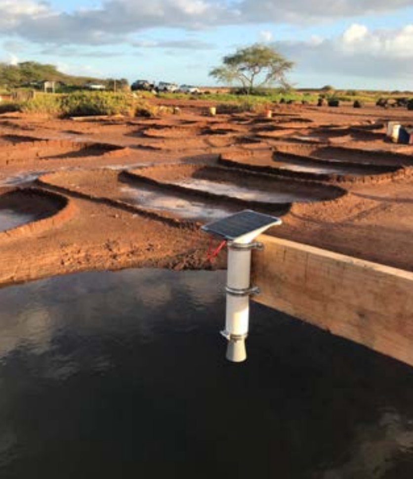
Figure 7. Photo of water level sensor deployed over a puna (dug well).
