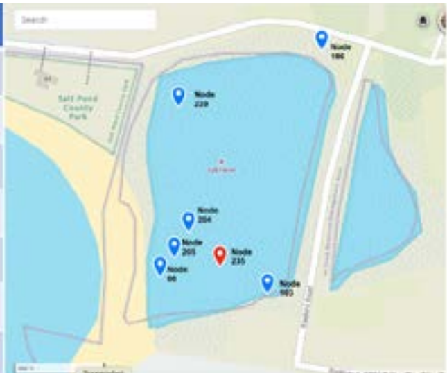
Figure 8. Image of individual water level sensor locations in Salt Pond, which were installed on site by Hui members, in consultation with UH researchers. Specific installation locations were selected for highest priority locations, as determined through consultation between Hui members and UH researchers. More information on sensor sites and installations are available in Appendix 1 and at: https://www.gaiagps.com/public/RcYcxuc1cuHNDw2J2rqIXGzF .
