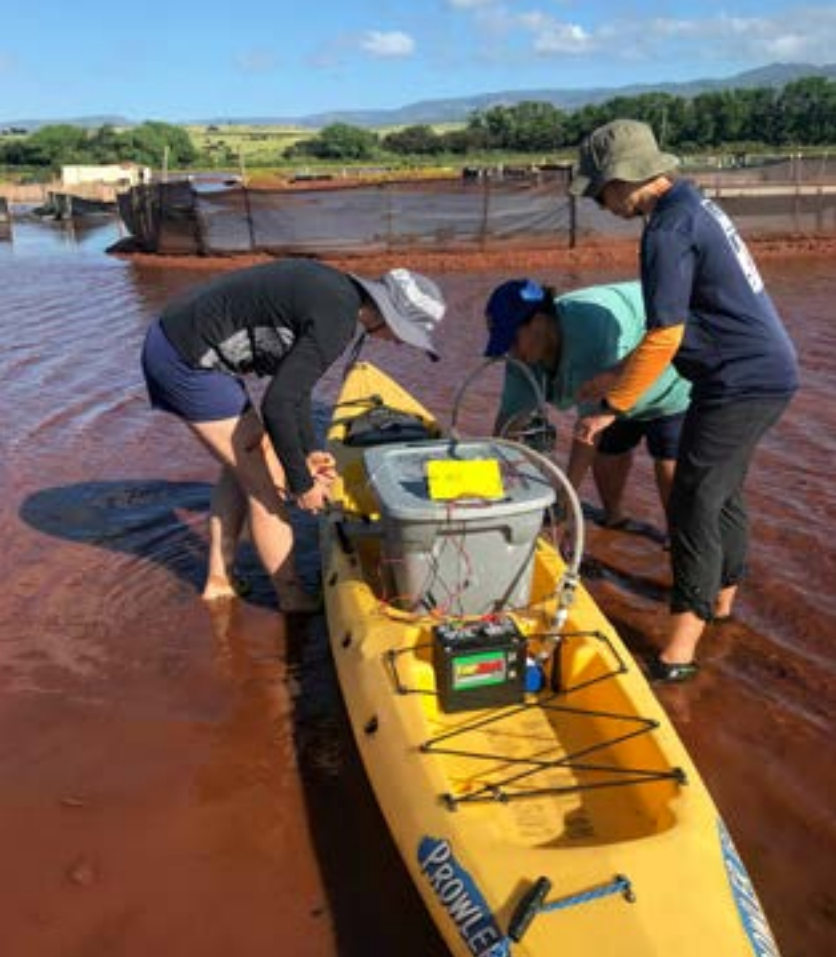
Figure 10. Photograph of the spatial survey researchers in the pond with the kayak and the RAD-Aqua with CTD Diver equipment.
