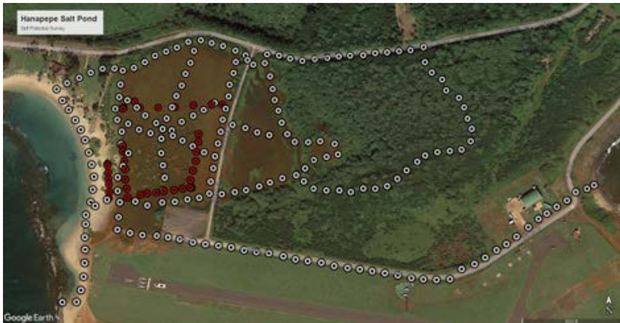
Figure 23. Geophysical Survey Map. Shown in white are the locations of the self potential (SP) measurements. In red are the electrical resistivity tomography (ERT) lines, red dots indicate 10 m increments along the ERT lines.
