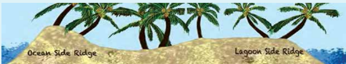
Figure 2-25. The ridges of an atoll serve the important function of protecting inland areas from wave inundation and flooding. Thus they should be maintained and enhanced if possible.
