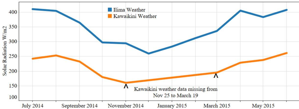
Figure 4. Monthly average solar radiation for monitoring period.
